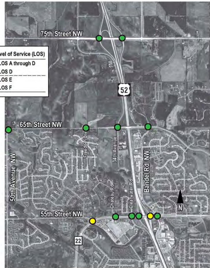
EXISTING CONDITIONS: PM PEAK HOUR TRAFFIC
